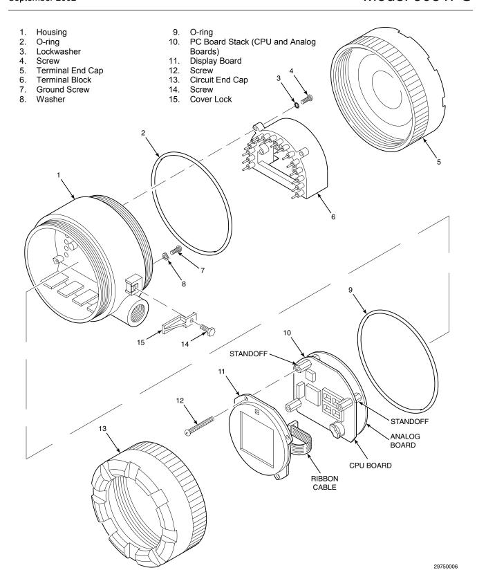
Figure 5-1. Two-Wire In Situ Oxygen Analyzer Exploded View
